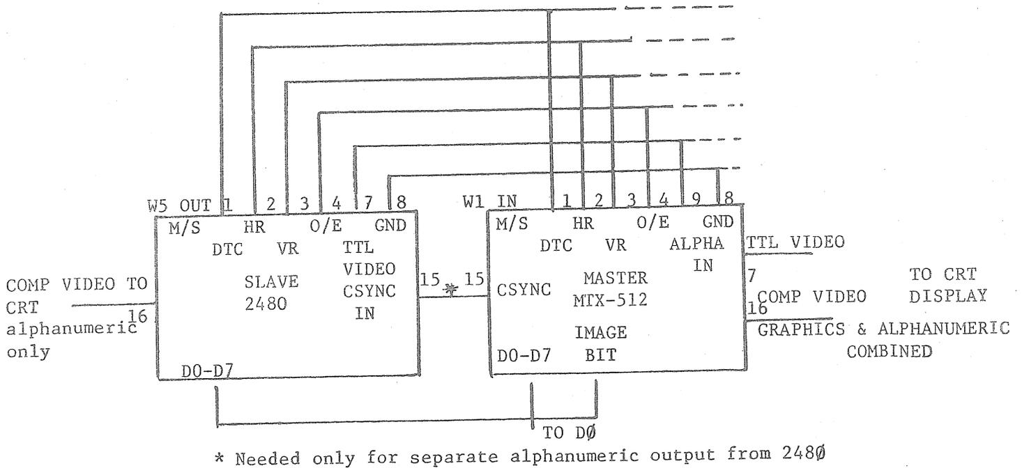
FIG 7 - ADDING 2480 and MTX-512 OUTPUTS FOR A COMBINED ALPHANUMERIC/GRAPHIC DISPLAY
