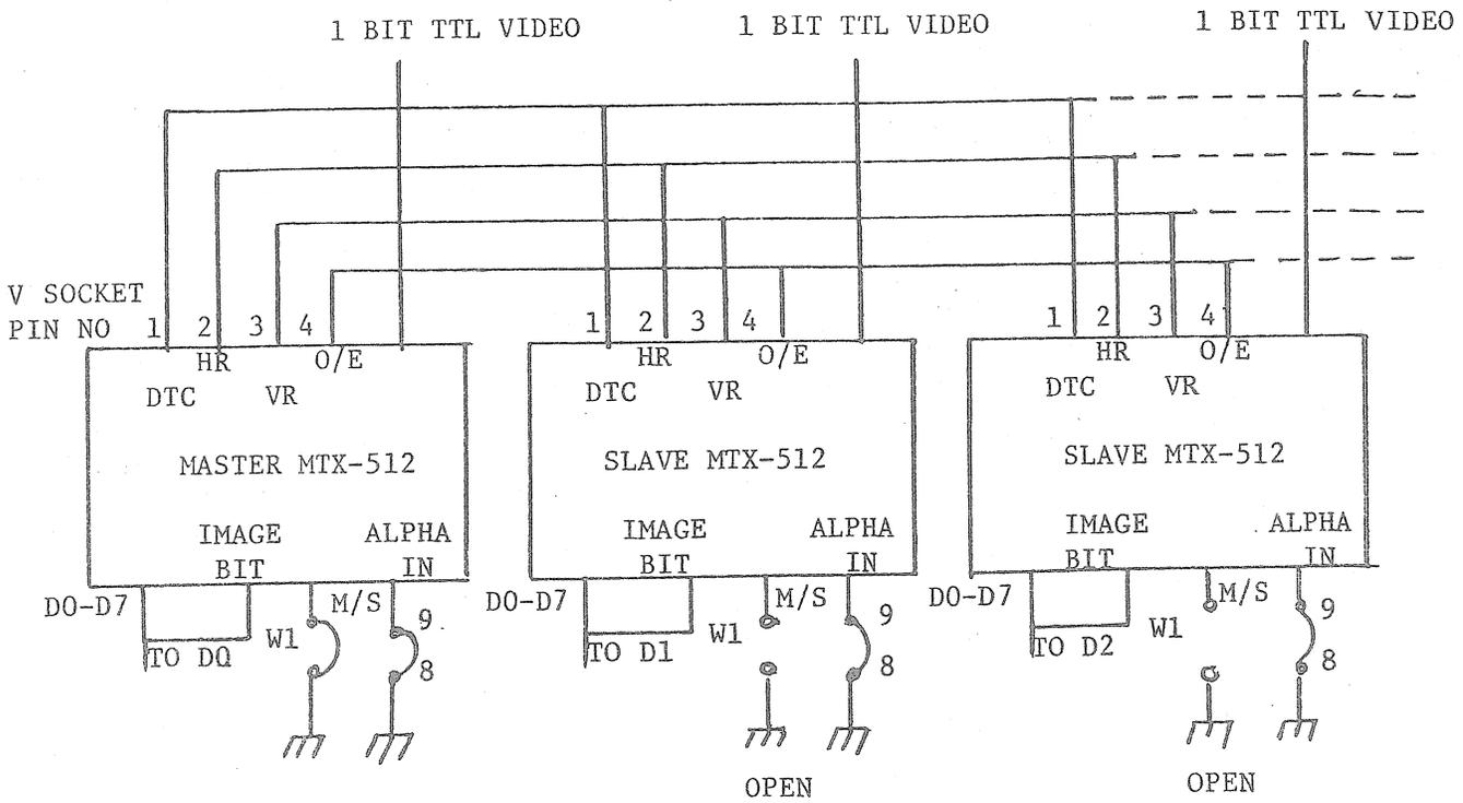
FIG 6 - SLAVING MULTIPLE MTX-512 CARDS FOR COLOR/GREY SCALE APPLICATIONS
