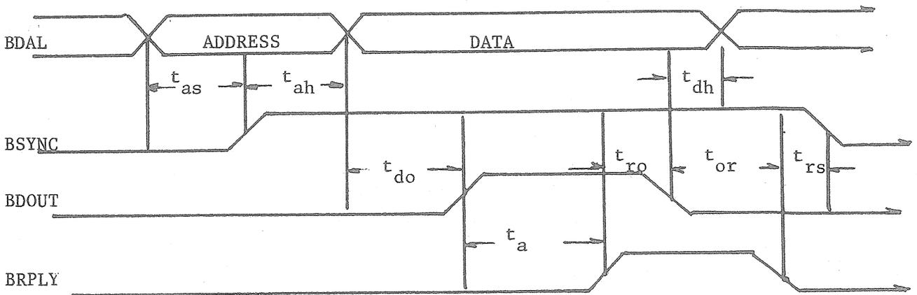
FIG 11 - DATA OUT (WRITE) CYCLE TIMING
