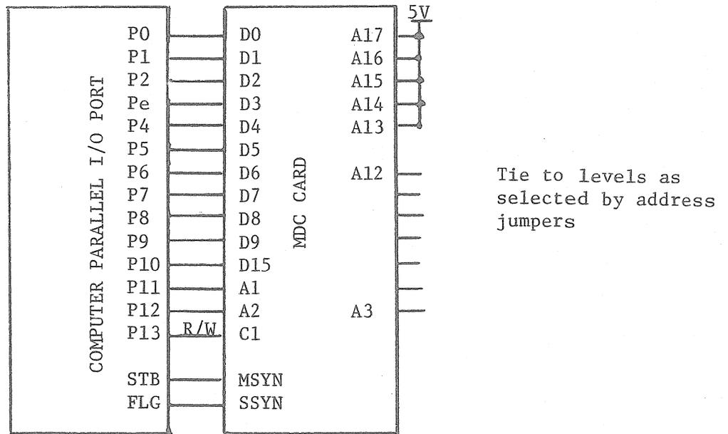
Fig. 9 - INTERFACING MDC CARD TO STANDARD PARALLEL I/O PORT
