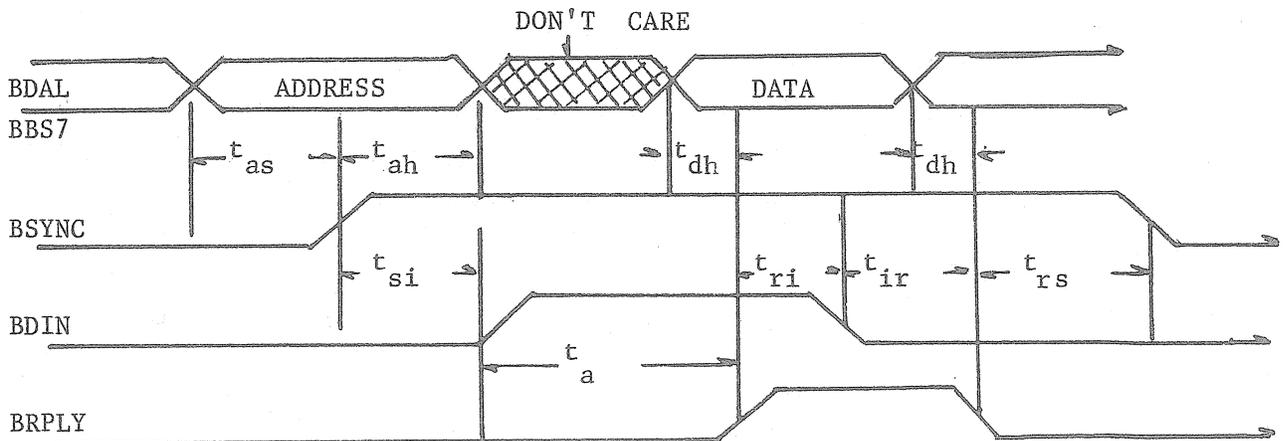
FIG 10 - DATA IN (READ) CYCLE TIMING
