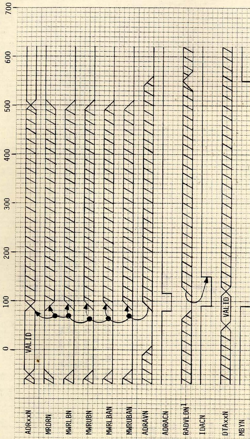
1 - During a Write Double Word, RADVLDN may occur at anytime. However, if it occurs later than 65 nanoseconds after ADRAVN, IDACN will be delayed by an equal amount. If RADVLDN occurs later than 195 nanoseconds after ADRAVN, MBYN will be extended an equal amount, thus increasing the cycle time of 550 nanoseconds.
